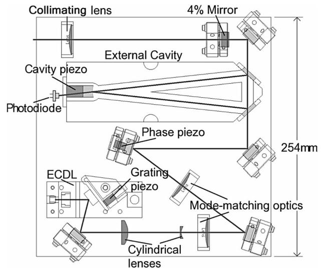
Fig. 1. Schematic of the laser setup with a superimposed laser beam.
