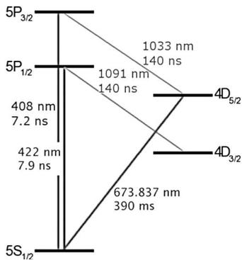
Fig. 4. Diagram of the relevant states of  $\text{Sr}^+$ .
