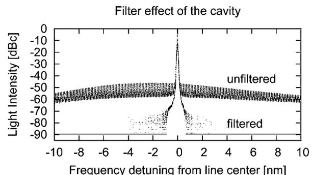
Fig. 3. Spectrum of the 674 nm laser at the ECDL (top trace) and after the filter cavity (bottom trace).  $-90$  dBc indicates null intensity.
