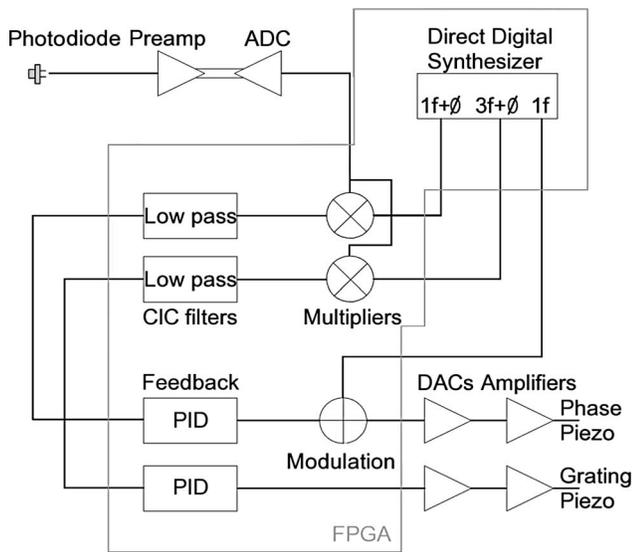
Fig. 2. Schematic of the digital lock system. The gray box denotes components implemented digitally using a field-programmable gate array (FPGA).
