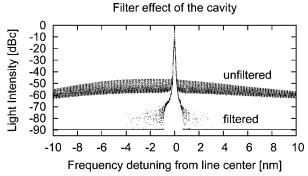
Fig. 3. Spectrum of the 674 nm laser at the ECDL (top trace) and after the filter cavity (bottom trace). –90 dBc indicates null intensity.
