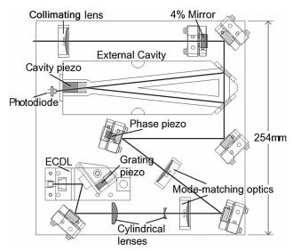
Fig. 1. Schematic of the laser setup with a superimposed laser beam.
