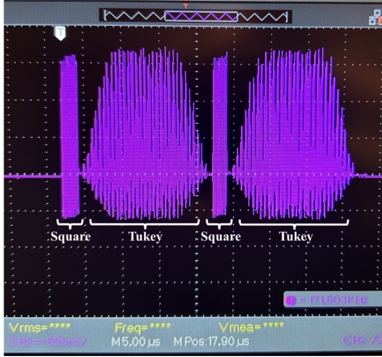
Figure 3.18: Screenshot of a photodiode signal of the 355 nm inner arm beam at low power. The pulse sequence is labeled on the image and consists of square and Tukey-like pulses. The sequence mimics a Trotter sequence of interweaved single and two-qubit gates. The light pulses are shaped (or amplitude modulated) by the Phaser as outlined in the text. The photodiode averages over the individual light pulses; oscillations and the vertical asymmetry are artifacts.
